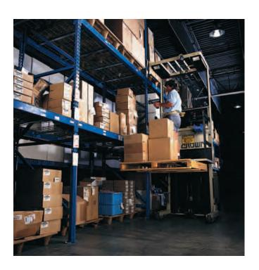
another worker, high in the air, picking an order using a vehicle-mounted bar code reader.
