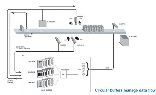
If the system acquires images faster than it can process them, filling up the buffer space, the frame grabber can deposit the extra image data in a special frame buffer called the "trash buffer." The system can then initiate a hardware event, indicating that there is image data in the trash buffer that must be monitored. As a partial recovery, the application software can read the image's time stamp, track that object through the system and assign it to the "not inspected" bin.
