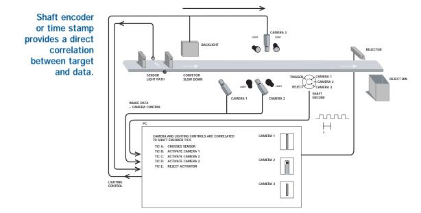
Because there is a time lag between image capture and analysis, the time stamp ensures that the system always acts on the correct target. The time stamp can also help with long or high-speed image sequences, where analyzing the time interval between images can determine if an image was missed during the capture sequence.
